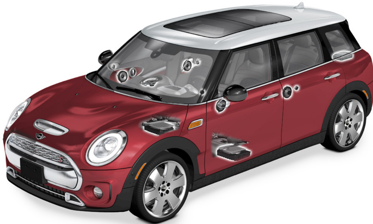
674- Hi-Fi loudspeaker system harman/kardon (12 speaker system with DSP amplifier) layout
